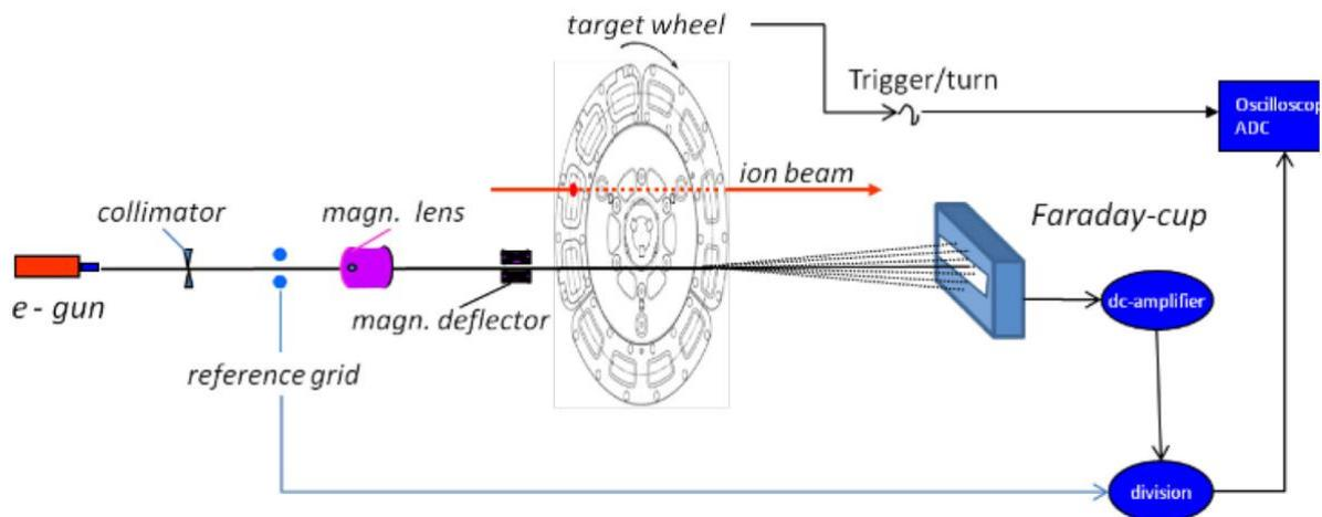
Figure 1: **Scheme of the electron gun with associated electronics and target wheel [4].**
