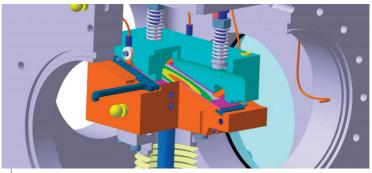
1 kW irradiation station for R&D on methods of production of innovative radioisotopes. Constructed and tested by the Nuclear Physics Institute of the Academy of Sciences of the Czech Republic, this station will be operated in the Neutrons For Science converter room. The green, yellow and red ellipses represent the impact of the beam on the inclined target.
